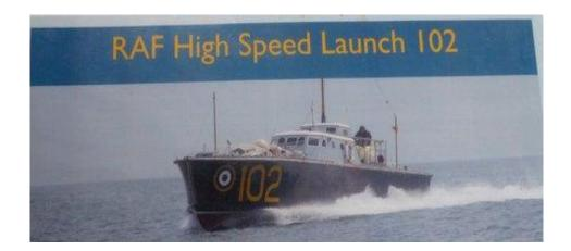
HSL 102 was built in 1936 by the British Powerboat Company of Hythe and probably one of the first fast offshore rescue boats in service with the RAF ASR in 1937. Her hull was made from African mahogany of double-diagonal construction and powered by three Sea Napier petrol engines which gave her a speed of 38knots. During her restoration these were replaced by three six-cylinder 420bhp Cummins diesels. She is the only 100 HSL to survive.
