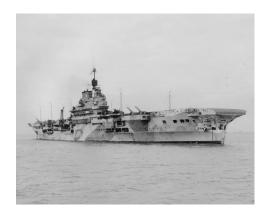
Class and type: Modified Illustrious-class aircraft carrier Displacement: 23,000 tons standard, 29,730 tons loaded
